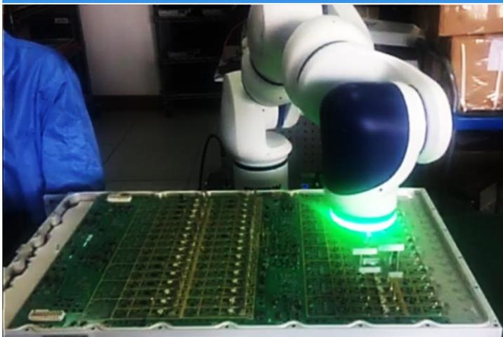
PCB board pin inspection
