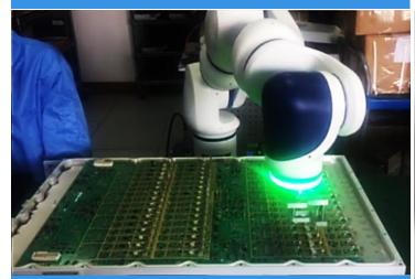
PCB board pin inspection
